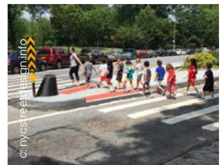
Figure 3.12. Median crossing reduces the crossing length and exposure to vehicle traffic for pedestrians.
