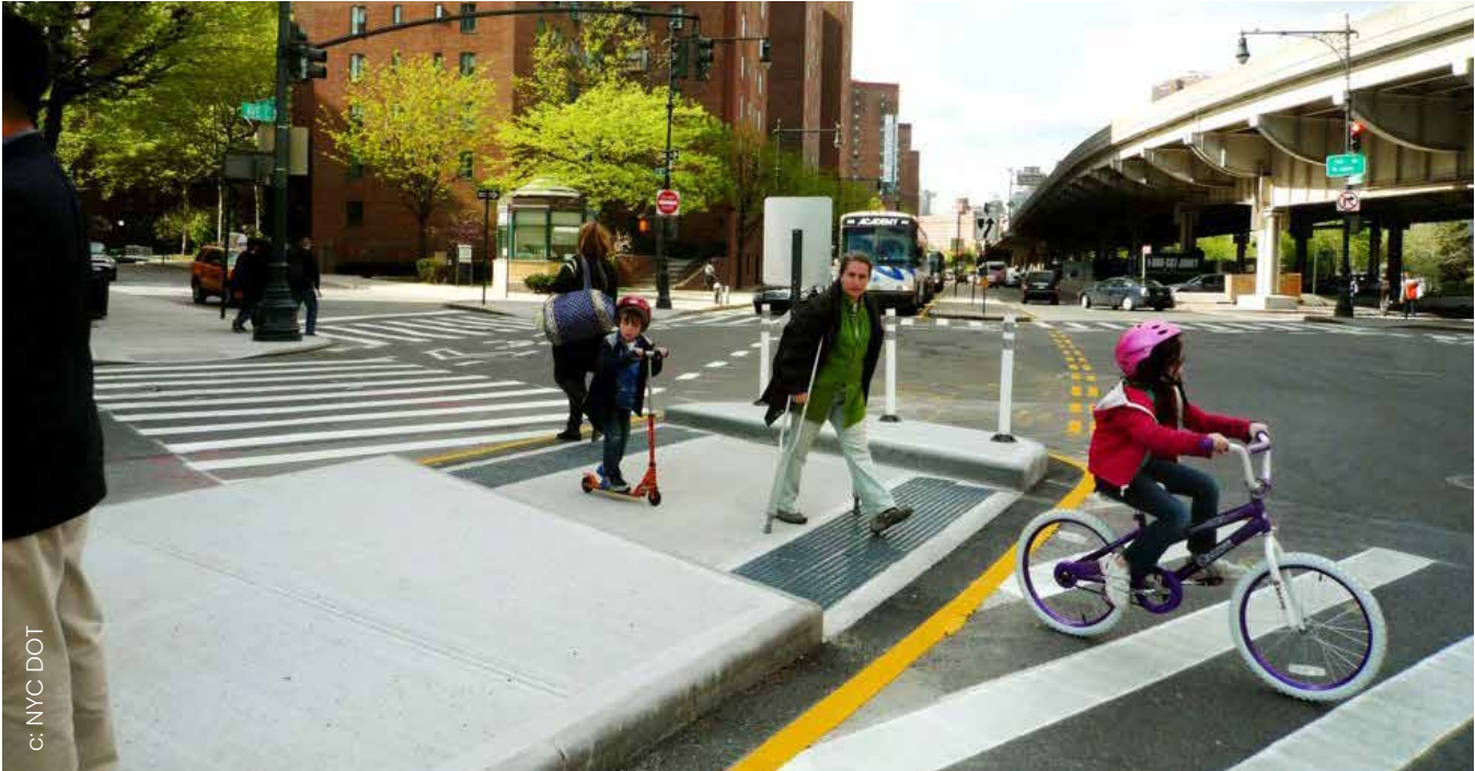
Figure 4.55. Refuge islands in the centre of wide streets with high traffic volume locations reduces the exposure time experienced by a pedestrian in an intersection.
