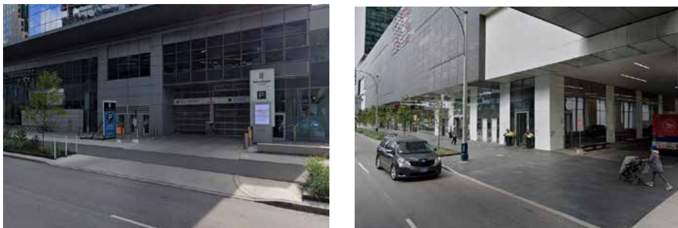
Figure 4.37. Two examples of raised driveways that emphasize safe pedestrian and cycling movements over turning vehicles. On the left is a high volume parking garage entrance with pedestrian clearway and bi-direction cycle track. Note how the arrangement of materials de-emphasizes the turning radii. On the right is the primary parking and service entrance for a large urban development. Note how the boulevard materials continue through the driveway to make clear to motorists that they are not the priority in this space.
