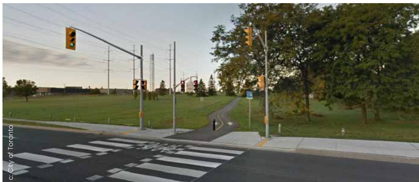
Figure 3.20. This image demonstrates how to consider the desire lines of trail users who want to cross a busy street. Providing a signalized junction with markings makes the connection more safe and convenient.
