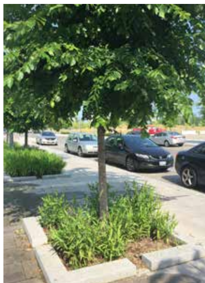
Figure 4.62. Street trees should have appropriate spacing and soil volume.
