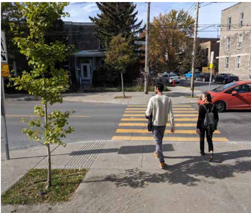
Figure 3.11. Curb extensions increase the overall visibility of pedestrians by reducing the crossing distance for pedestrians
