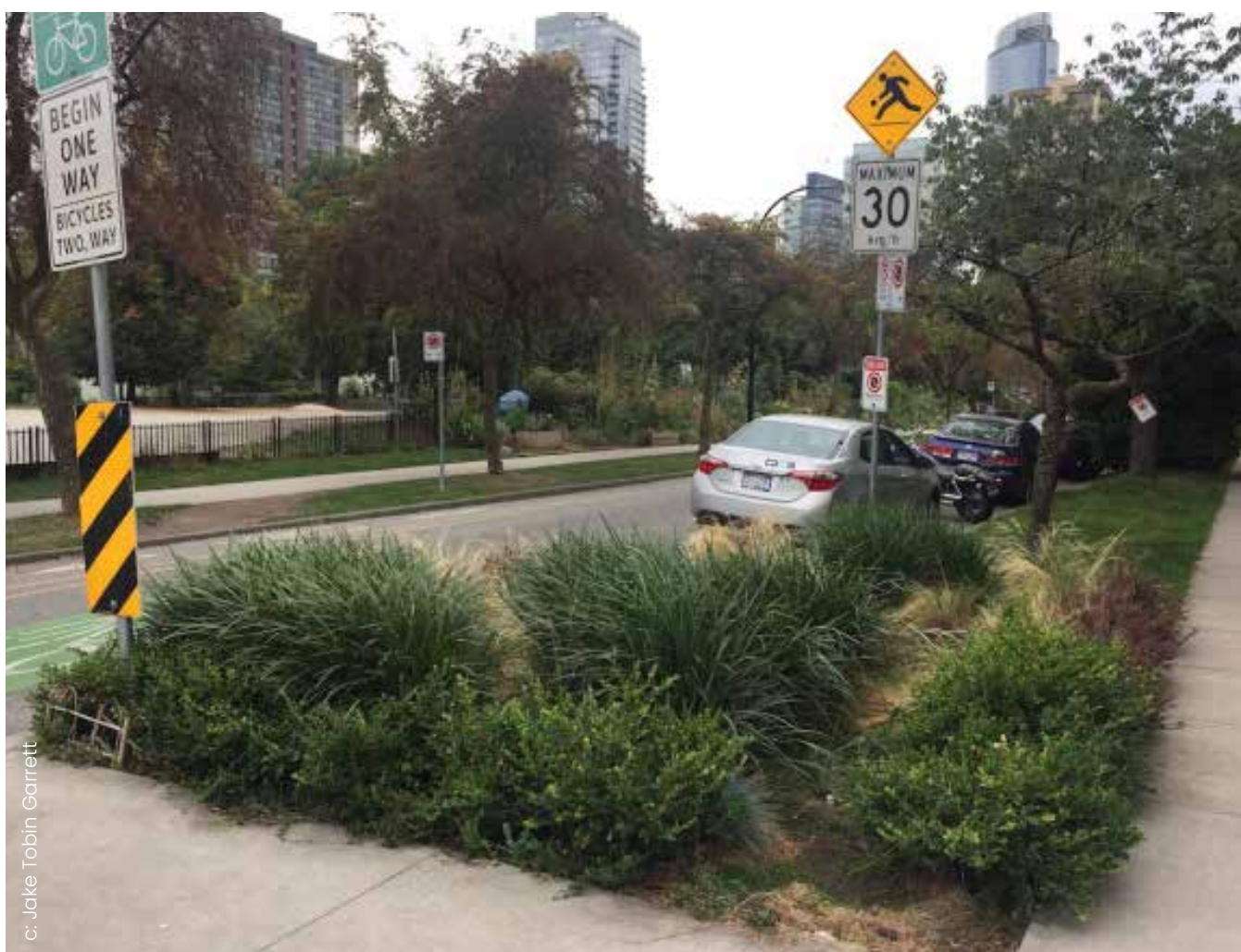
Figure 3.29. Storm water management techniques are possible in many different street types and parts of the right of way, and can contribute to place making and traffic calming.
