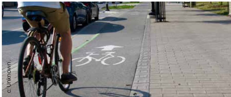
Figure 4.20. Cycling tracks separated from the pedestrian clearway through a change of paving material.
